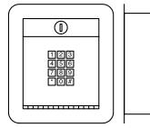
**1503/06 Flush** keypad with trim ring: 7.125" W x 8.375" H x 4" D 305mm W x 343mm H x 63.5mm D rough-in box: 5.625" W x 7" H x 4" D 305mm W x 343mm H x 63.5mm D
